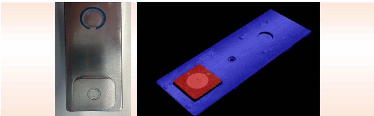
Six-surface defect detection of the lithium battery (scratches and dents)
