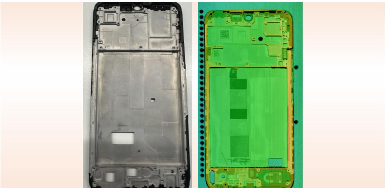
Height measurement of precision parts step
