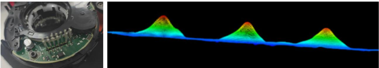
Height detection of the PCB parts
