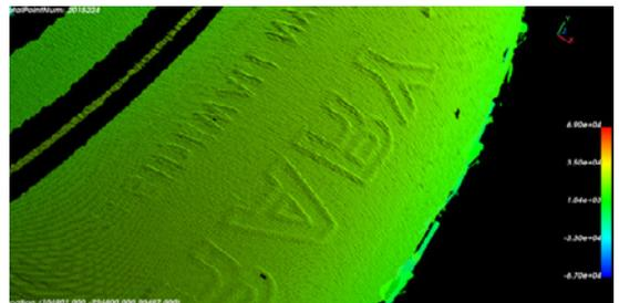
Weld bead defect detection of bearings
