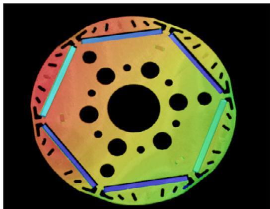
Defect detection of structural part welding seam
