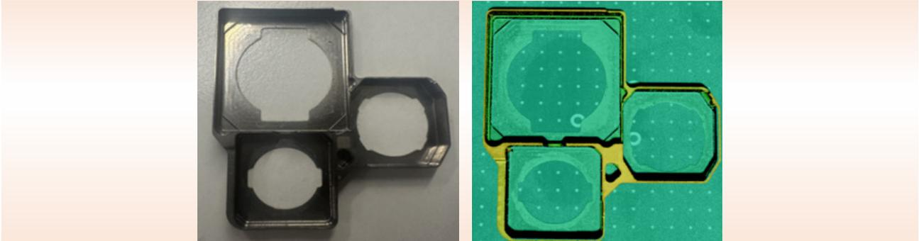
Measurement of step and flatness of mobile phone card slots
