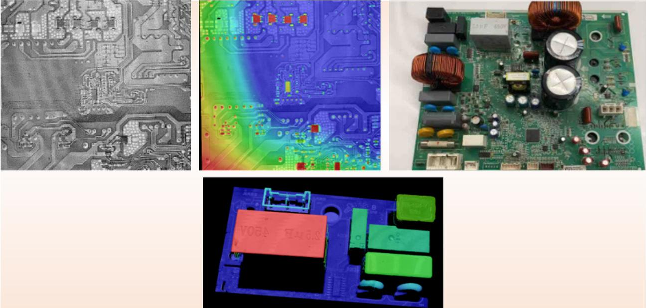
Measurement of soldering height and volume
