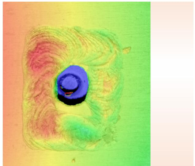
Defect detection of the tab welding
